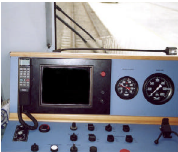
Figure 2 – CargoSprinter Driver's Desk
