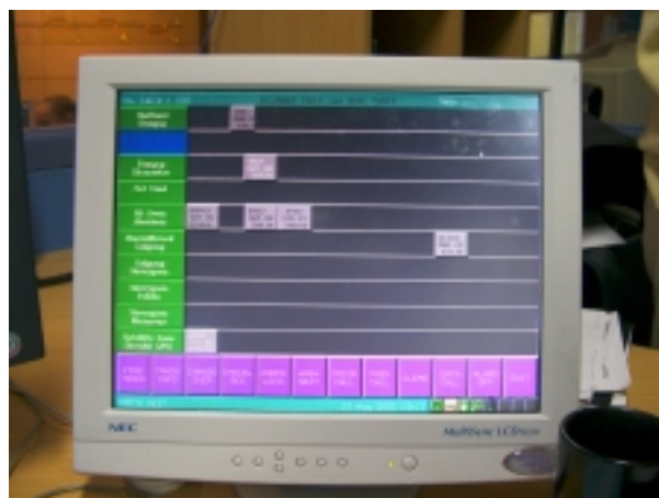
Figure 6 : Countrynet Train Controller Workstation – train locations (grey squares) are plotted from the GPS data
