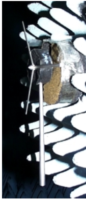
Fig. 6. Wind turbine scaled model placed on the chamber azimuth positioner.
